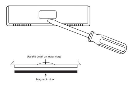
Gently slide a screwdriver into the bottom edge of the badge. Gently turn the screwdriver counter clockwise. The badge is held on by a magnet in the well of the battery door. The badge should pry off easily. DO NOT USE FORCE.
