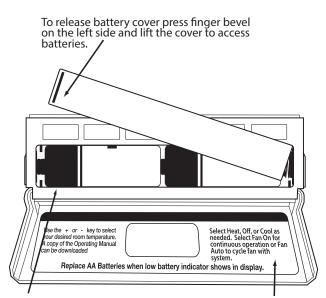
Insert 2 AA Alkaline batteries (included). High quality alkaline batteries are recommended.
