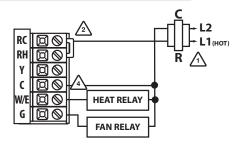
In many systems with no emergency heat relay a jumper can be installed between E and W2.
