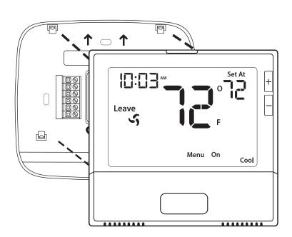
Align the 4 tabs on the subbase with corresponding slots on the back of the thermostat, then push gently until the thermostat snaps in place.
