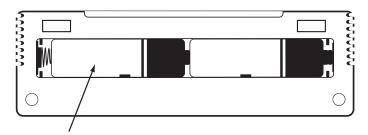
Insert 2 AA Alkaline batteries (included) located in the back of the thermostat. High quality Alkaline batteries are recommeded.
