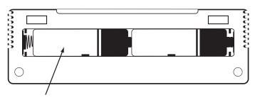
Insert 2 AA Alkaline batteries (included). High guality Alkaline batteries are recommneded.
