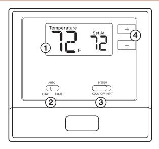
1LCD3System Switch2Fan Switch4Temperature Setpoint Buttons
