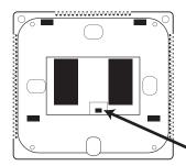
**Gas**: For systems that control the fan during a call for heat, put the fan operation switch to the GAS position. **Electric**: For systems that do not
