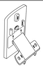
2 T-bracket will stop on the top of the slot holders.
