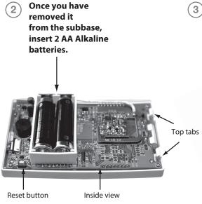
Attach the thermostat to the subbase by aligning the two top tabs and then close as shown.
