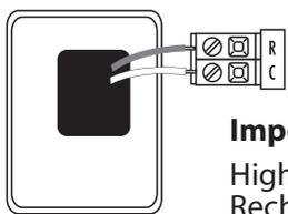
Battery installation is optional if thermostat is hardwired (R and C terminal connected to 24V power).
