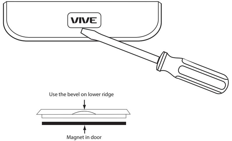
Gently slide a screwdriver into the bottom edge of the badge. Gently turn the screwdriver counter clockwise. The badge is held on by a magnet in the well of the battery door. The badge should pry off easily. **DO NOT USE FORCE.**
