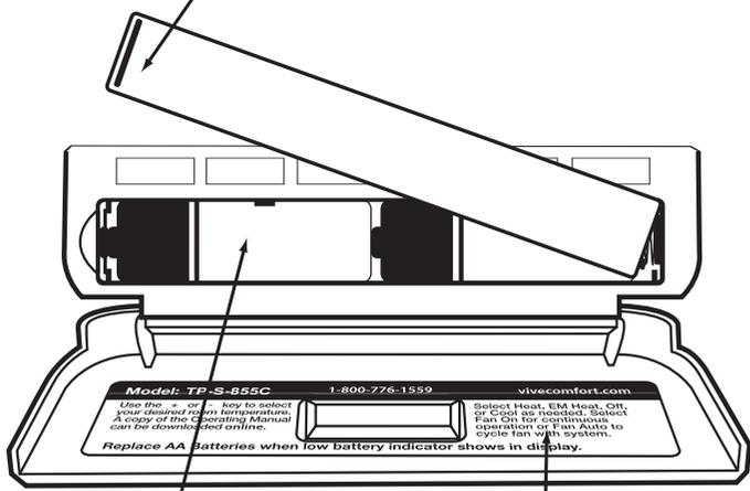
Insert 2 AA Alkaline batteries (included). High quality alkaline batteries are recommended.
