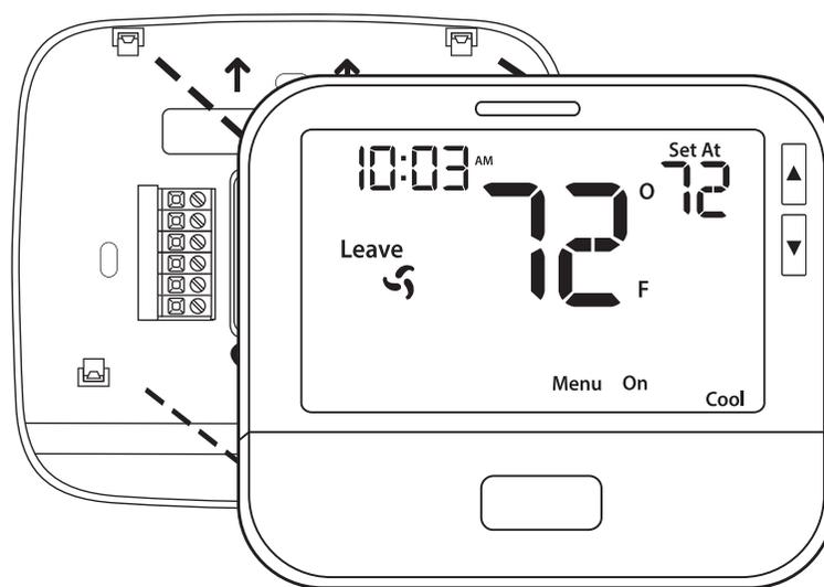
Align the 4 tabs on the subbase with corresponding slots on the back of the thermostat, then push gently until the thermostat snaps in place.
